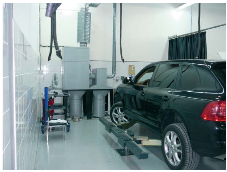
High vacuum filtering unit with spark protection monitoring (500 m³/h) for 2 aluminium workplaces in the body repair shop.
