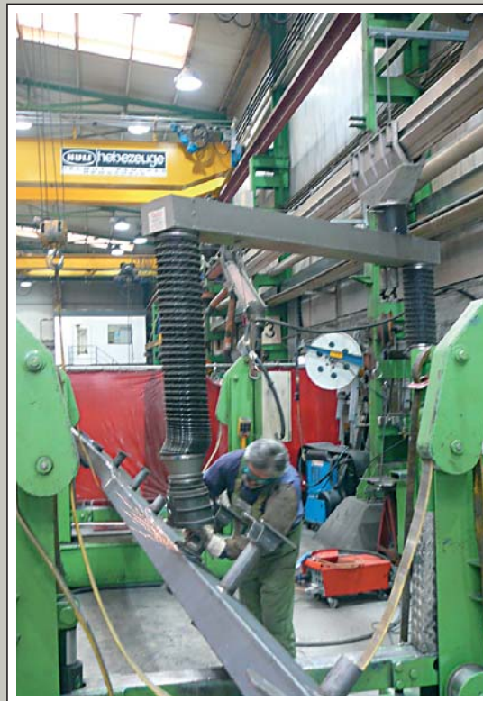
Aluminium rail system type SSK 290 with moving trolley and a extraction telescope arm for welding and grinding in a industrial workshop with long pieces.
